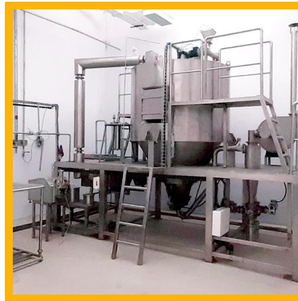
Pilot Scale Dryer 10 litre per hour
