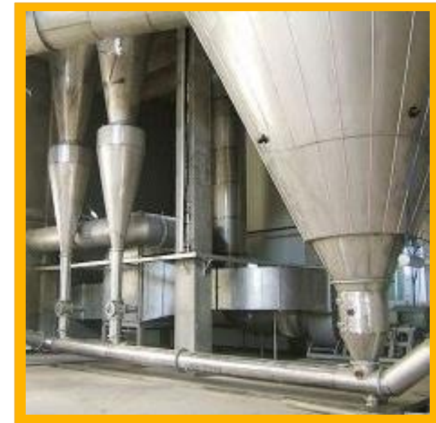
Commercial Scale Dryer 800 kg per hour
