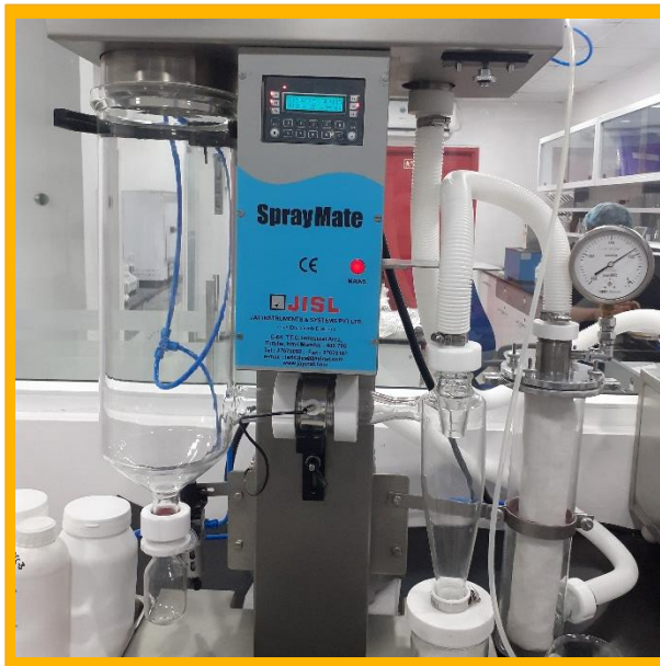
Lab Scale Dryer 1 litre per hour
